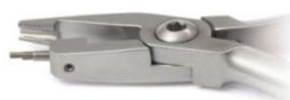
IH504 Loop forming plier Tweed style For round and rectangular wires. Replaceable cylindrical beak with three sizes: 0.045" (1.14 mm); 0.060" (1.52 mm); 0.075" (1.90mm)
