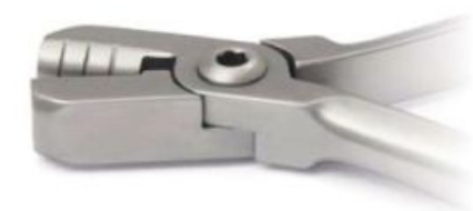
MIH509 Arch forming and contouring plier For wires of 0.016" (0.41mm); 0.018"(0.46mm); 0.022" (0.56mm)
